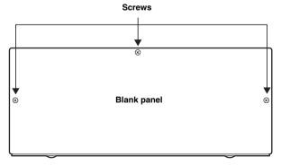
Take care not to catch the internal wiring when reattaching the panels.
